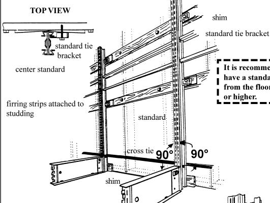
It is recommended to have a standard tie bracket 30"-36" from the floor when the standard is 108' on higher
