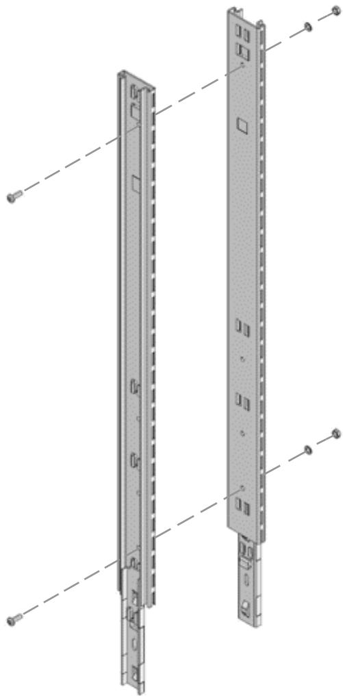
To assemble a center standard extender take two (2) end extenders put them back-to-back and secure with two (2) 1/4-20 x 3/4 screws (one top and one bottom as pictured), two (2) 1/4 washers, and two (2) 1/4-20 hexnut.
