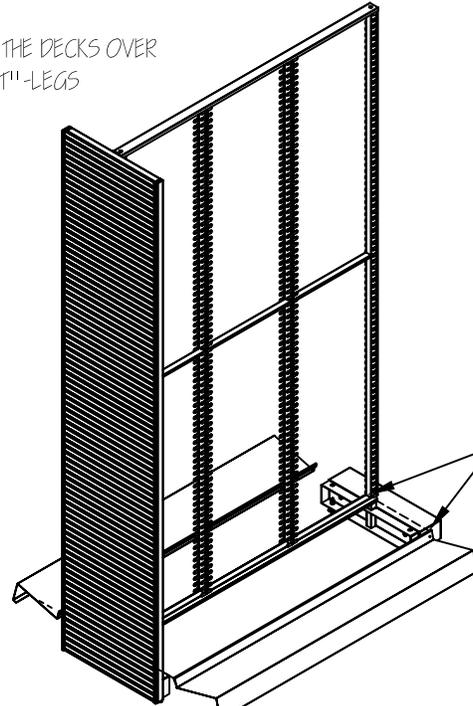
HOOK THE METAL DECK TO THE FIRST UNIWEB RIB
