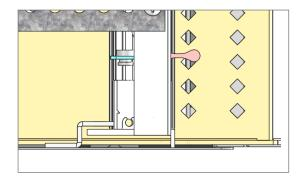
Read step 6 before continuing. Install the door assembly by engaging the sides of the door assembly into the "S" shaped groove of the end panels. You may need to tip the top shelf to clear the door assembly. See the figures on this page. Some items not pictured for clarity.
