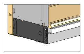
Secure the end panels to the deck using a #10-16 x 3/4 TEK screw.
