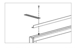
Secure the strap and gap filler to the door assembly using (2) #10X1/2 sheet metal screws. See the illustrations on this page for proper installation.
