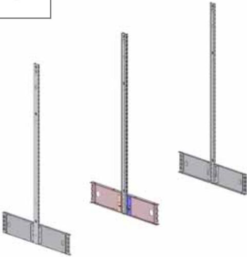
With the left upright (smooth side out) in hand, take the left hand bottom arm (smooth side out) then slide it into the upright and push down to seat the hooks.
