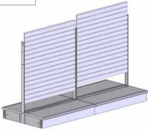
Install the slatwall back panel by inserting it into the channels slightly above the tie bar and slide it down the channels on the uprights as shown to the left. When installed the slatwall back panel should rest in or on the cross tie channel as shown below.
