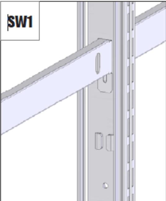
Install the slatwall tie bar by sliding it into place as pictured to the left. You may need to tap the slatwall tiebar to properly secure it.
